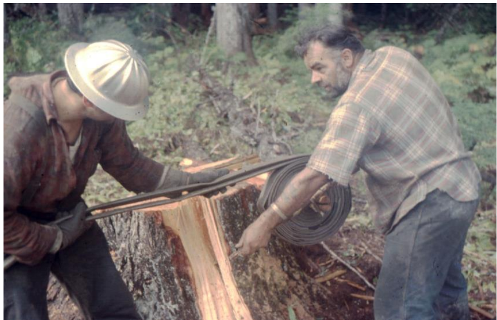
The ingenuity of these logger/ firefighters in the design and manufacture of this wilderness model wet fire hose roller.
