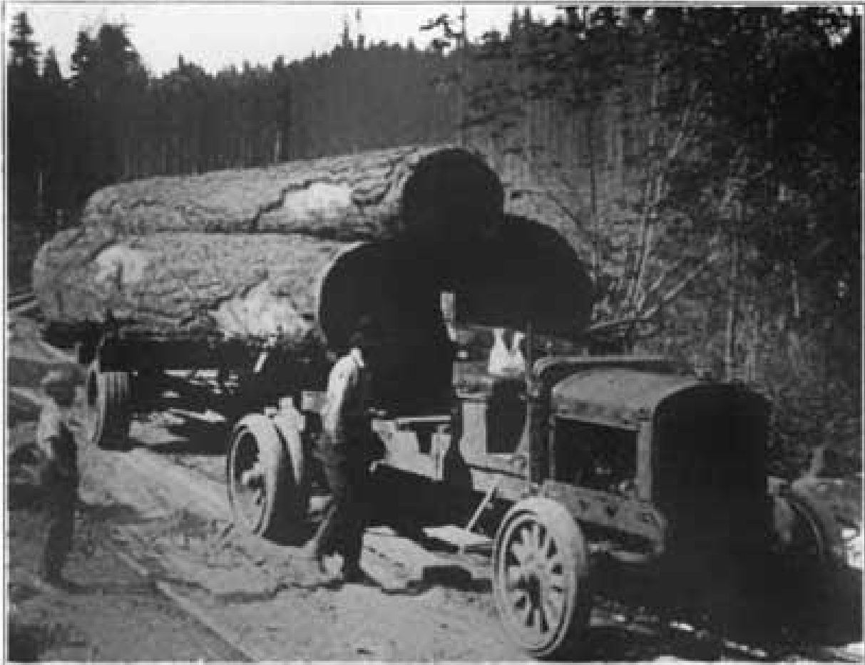
A 5-TON GENERAL MOTORS CO. TRUCK AND 8 \frac{1}{2} -TON PACIFIC CAR & FOUNDRY CO.'S DOUBLE BUNK UNIVERSAL TRAILER, LOADED AND READY TO MOVE DOWN THE MOUNTAIN, A DISTANCE OF A MILE AND A HALF, THE ELEVATION AT THE LOADING POINT BEING 1200 FEET HIGHER THAN AT THE WHARF, WHERE THIS LOAD OF LOGS WILL BE UNLOADED: 5,500 FEET B. M. OF FIR LOGS ON THE TRUCK AND TRAILER.
